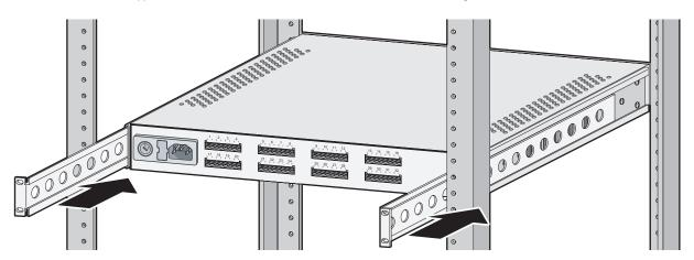
Figure 6. Inserting the Rear Support Rails
